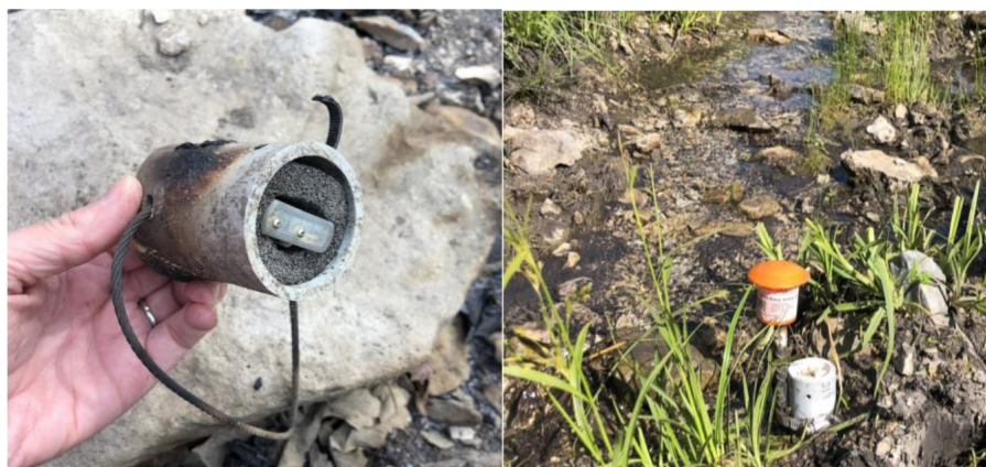
Figure 12. Monitoring inundation regimes is increasingly possible via in situ sensors. Pictured are stream temperature, intermittency, and conductivity sensors (STICs) (Chapin et al., 2014), one of the types of increasingly available sensors to measure water presence/absence in an inexpensive and easily deployable manner. These sensors can be used across all types of VIEs. Credit: Amy Burgin.
